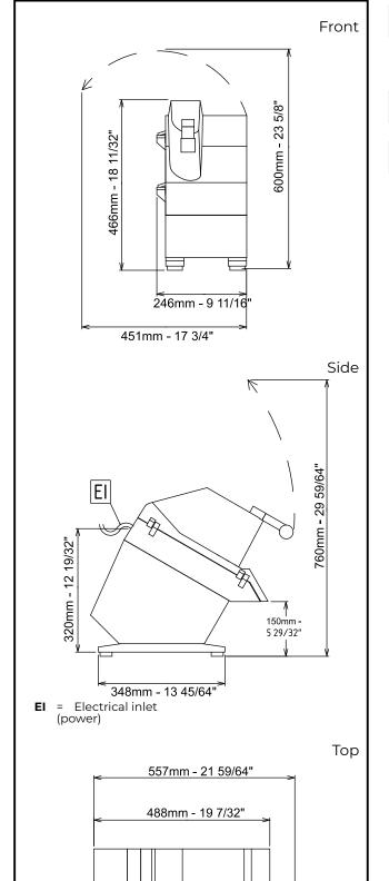
Electric 220-240 V/1N ph/50 Hz Supply voltage: Electrical power, max: 0.37 kW 0.37 kW **Total Watts:** Capacity: Performance (up to): 400 kg/hour Key Information: External dimensions, Width: 246 mm External dimensions, 557 mm Depth: External dimensions, Height: 466 mm **Shipping weight:** 21 kg
